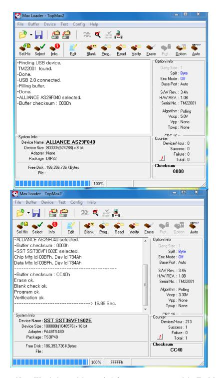
Note: Watch the model name in left-up corner screen and the TopMaxII won't be ready if "DEMO mode" appears in the screen. Check the USB cable and turn on the AC switch in the back side of unit.
